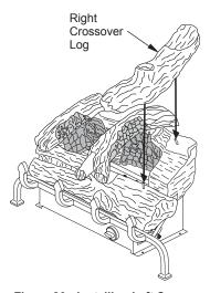
Figure 20 - Installing Left Crossover Log
